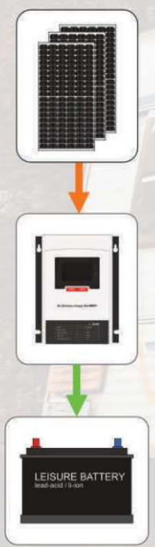
MPPT Charge the Leisure Battery
